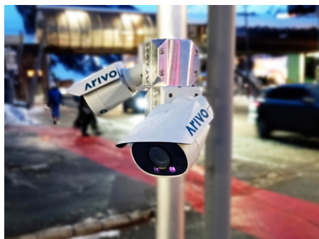
Arivo licence plate cameras capture the number plates of vehicles entering and leaving the city – reliably even in difficult weather conditions, according to the supplier.
