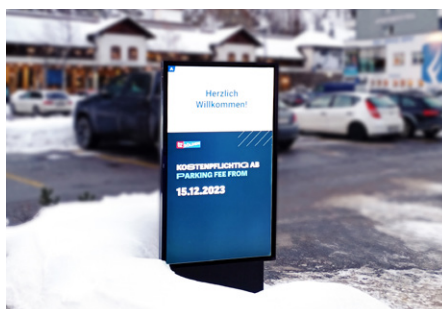
Information displays at the entrances indicate that the car parks are subject to charges. Entry displays provide live feedback that licence plates have been recognised – and exit displays indicate whether parking fees have already been paid.
